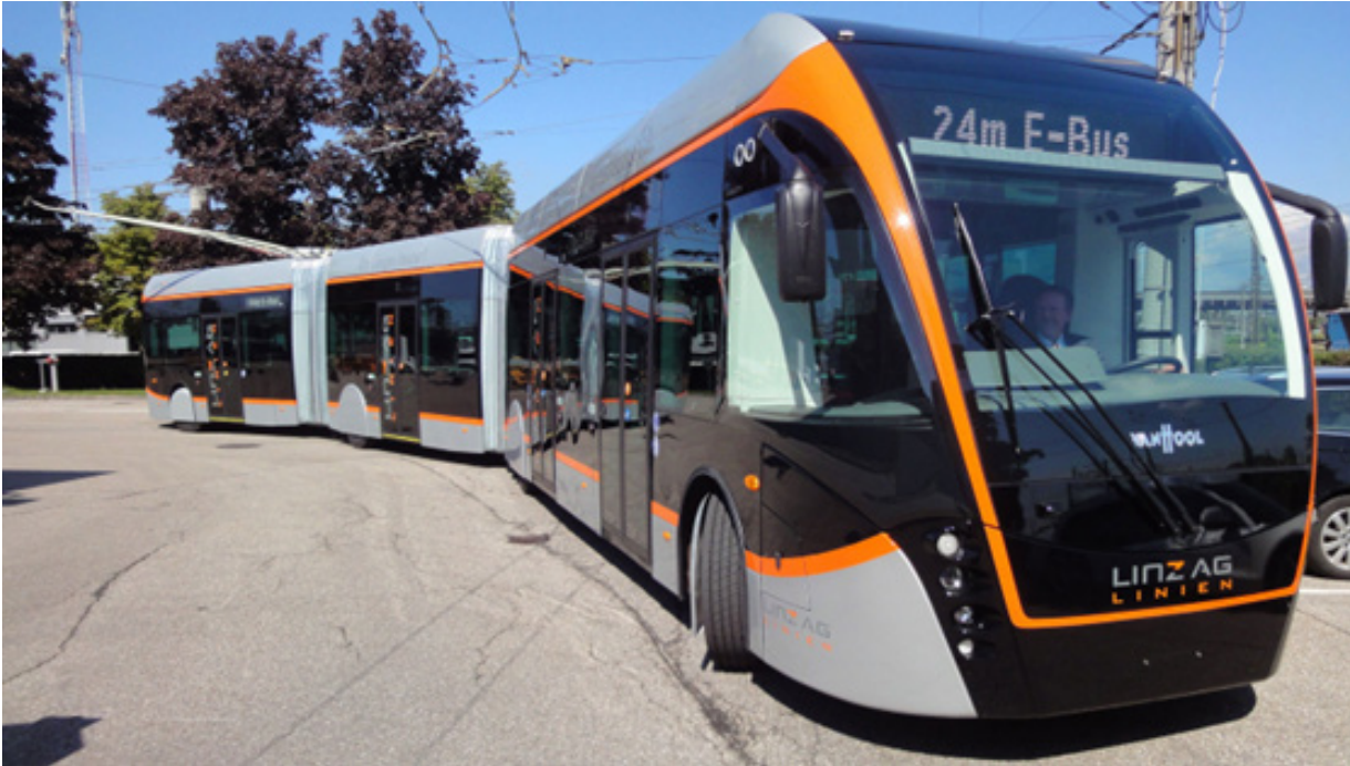
Picture: Double-articulated electric bus, Austria
