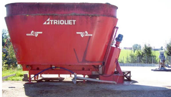
Hopper for dropping corn husks into methane digester – Germany.
